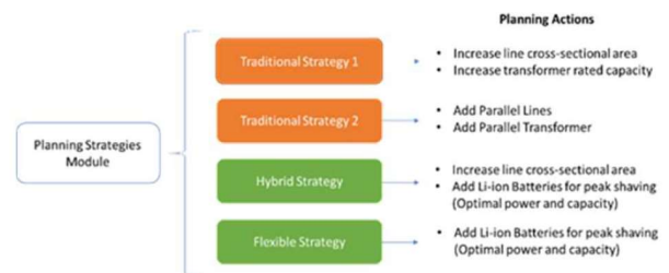
Fig. 44: Distribution planning strategies to exploit the use of Li-ion batteries (Paper 11016)
